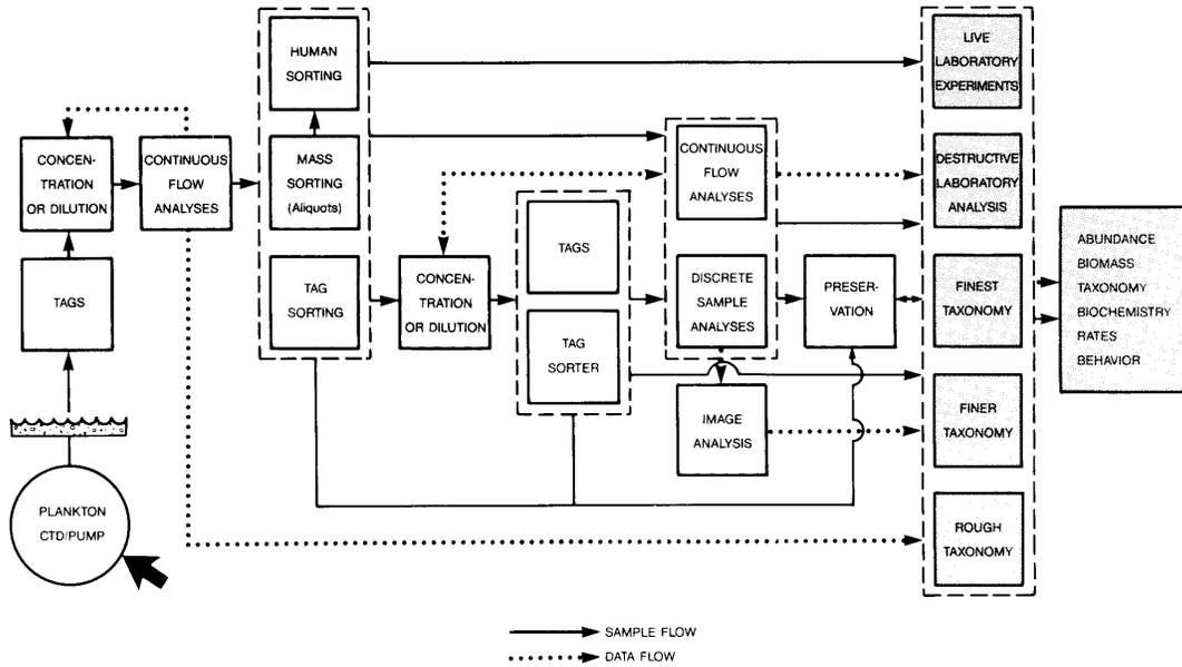
Figure 1. Basic components that would probably be integrated to comprise a shipboard automatic plankton analyzer system (SAPAS). See text for detailed description of figure.
