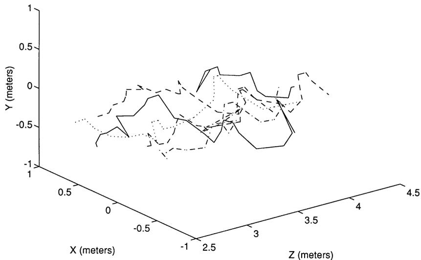
Figure 1. Six target tracks, reconstructed from an FTV sonar image.
