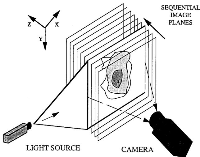
Figure 2. Components of the light stripe imaging system.
